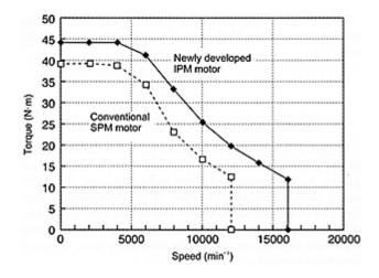
Fig. 2 Torque speed characteristics (instantaneous range: measurements actually taken) (input voltage: 3-phase, 200V, motor maximum current: 155Arms)
